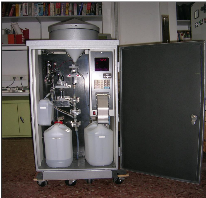
Figure 9: Kimoto AR-106 acid rain analyser installed at Torre Miró (1223 m).
